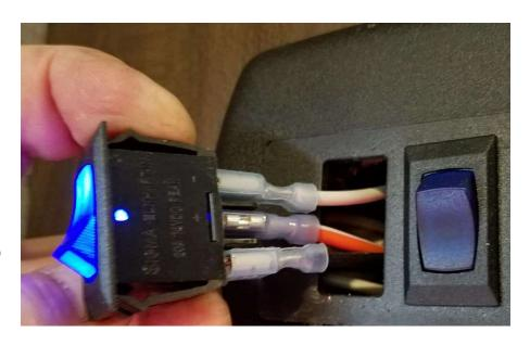
Every unit is likely wired differently but you should see three wires. A black, one of varying colors, and a white. On our camper... the white wire powered the blue laser light. On all of our light switches, it was the top wire, but I suspect that could vary.
