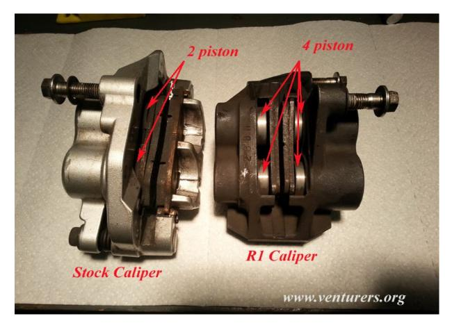
There are different styles of R1 calipers. Some that bolt up just like our stock calipers as shown above. Others however bolt on from the side instead of the front and are **NOT** what you want. These also have the gold star and will be listed as R1 calipers. But these **will not** work. See photo below.
