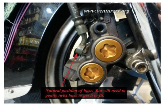
You could twist the line either clockwise or counterclockwise. Since I have chrome caliper covers, I twisted mine clockwise so the hose was bent in toward the fender. Be sure to position the line so you can still access your bleeder screw. After you connect the hose to the caliper you will need to twist and move the hose bracket so it aligns with the mounting screw location.
