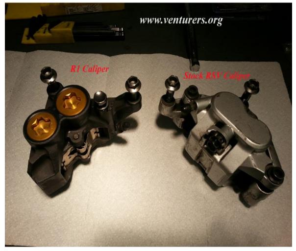
The stock calipers are a two piston floating style. The R1 are a fixed four piston design.
