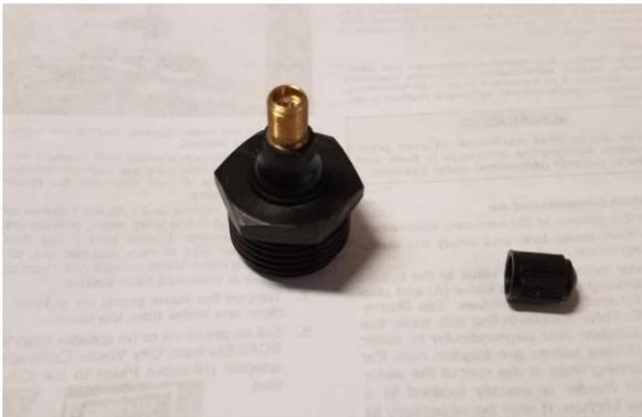
You will need an air valve plug similar to this in order to pressurize the water system to blow out the lines. I like this type as it has a Schrader valve and threaded nipple which allows my tire fill tool to attach without me having to stand and hold it on.
