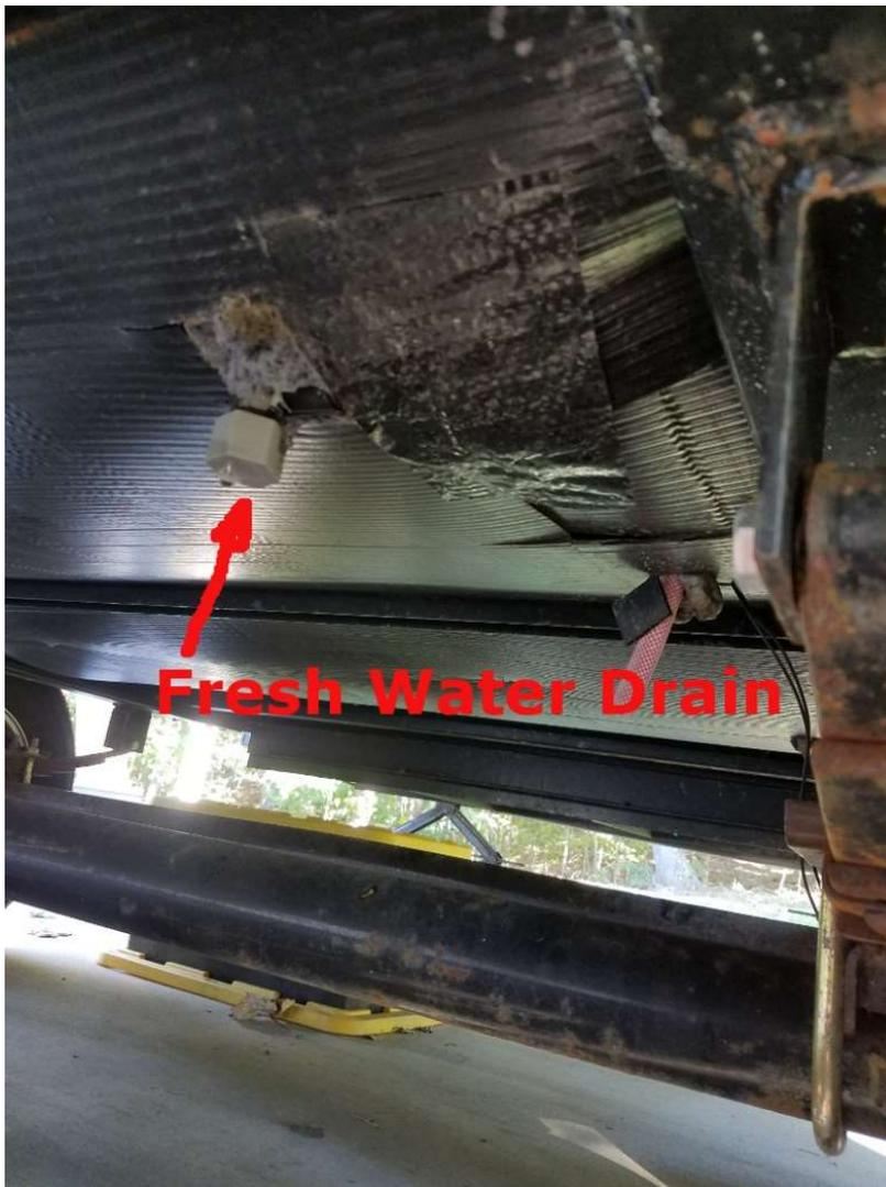
This is the location of the fresh water tank drain plug. It is located on the driver side just in front of the axles.
