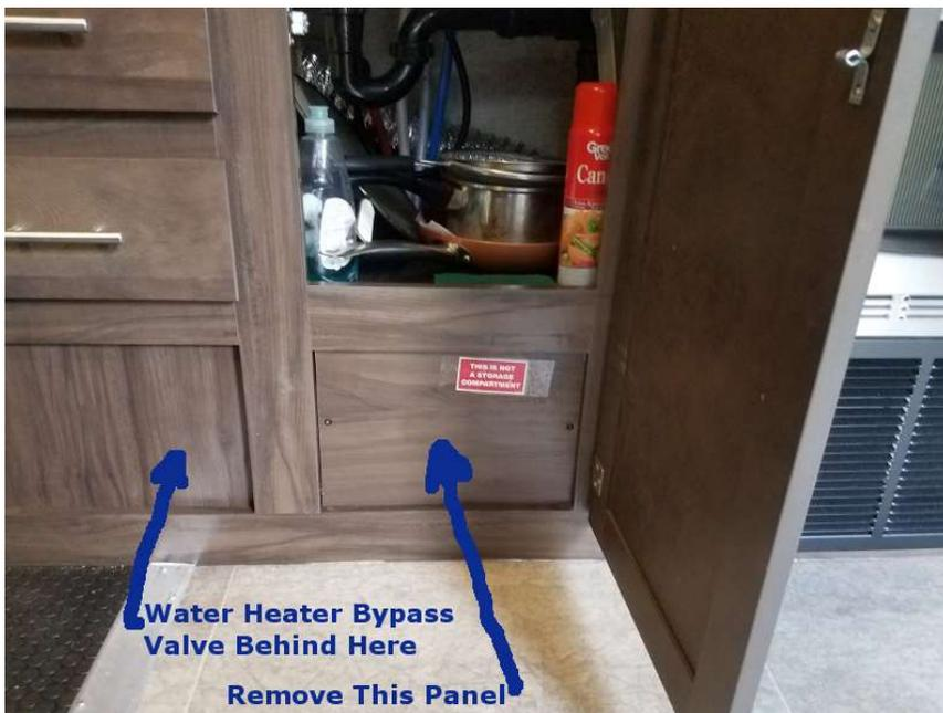
This is the panel in the kitchen that needs to be removed in order to access the hot water tank bypass valve and also the fresh water pump if you were doing the anti-freeze pumping method.
