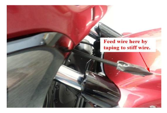
Next I decided to cut a notch in my top control panel in order to route the power and camera wires from controller to their locations. If you are not into cutting this notch, I suppose one could route the wires in the area between the fairing and forks. But I do not like this for two reasons. First I do not like any wires in that area that could maybe hang-up on forks causing me issues. Plus it would be sloppy looking to me.
