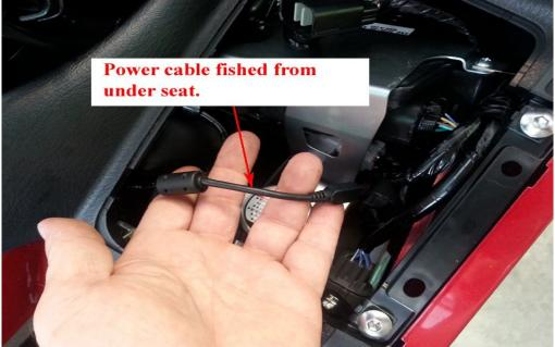
Next I fished the USB camera cable from the top right side control box area to come out under fairing. Again I used a stiff wire and taped the USB cable to it to fish through. Be careful to route wire so it does interfere with forks. One picture I did not take is where I routed the wire under the fairing to keep away from fork. There is a little sub-frame in the center of the fairing. I routed the USB in front of that to help keep it clear of forks. See photos:
