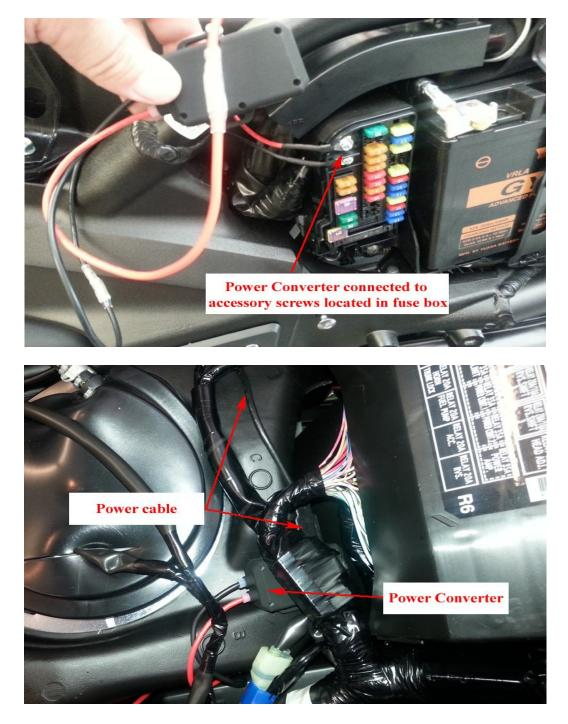
Next, route the power cable from the seat area to the upper right control panel area. I used a stiff wire and taped cable to it to fish under that top housing. See photos:
